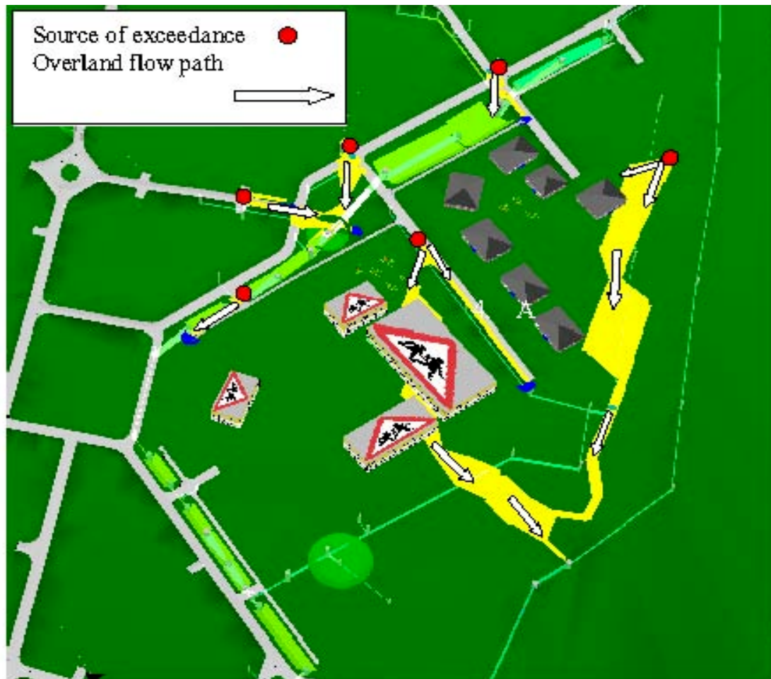
Figure 16.4 Flood flow paths for 100 year event with additional flooding due to climate change indicated by the lighter colour (courtesy MicroDrainage)
