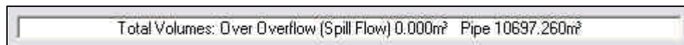
Figure 4.7 - Caption from the hydrograph tables in the Simulation module showing the pre-development runoff volume.
